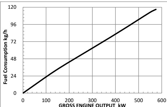
Curves shown above represent gross engine performance capabilities obtained and corrected in accordance with SAE J1995 conditions of 29.61 in. Hg(100kPa) barometric pressure [300ft.(91m) altitude] 77deg F (25 deg C) inlet temperature, and 0.30 in. Hg(1kPa) water vapor pressure with No.2 diesel or a fuel corresponding to ASTM D2.
