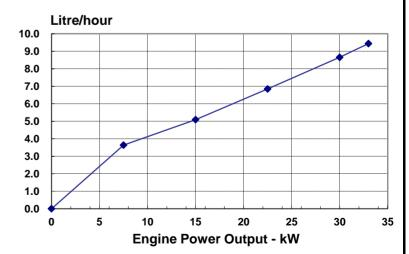
Curves shown above represent gross engine performance capabilities obtained and corrected in accordance with GB/T18297 conditions of 100kPa (29.61 in. Hg) barometric pressure [80 m (263 ft.) altitude], 25°C (77°F) inlet air temperature, and 1 kPa (0.30 in. Hg) water vapor pressure with No.0 diesel fuel.
