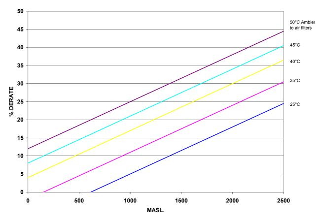
Note: Ambient temperature at air cleaner inlet.
